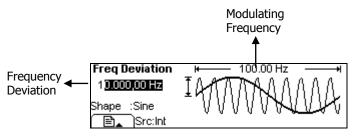
Figure 2-38 Waveform Parameter in the Graph Mode
