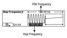
Figure 2-40 Waveform Parameter in the Graph Mode
