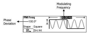
Figure 2-42 Waveform Parameter in the Graph Mode
