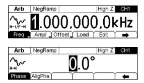
Figure 2-19 Arbitrary Signal Parameter Setting Interface
