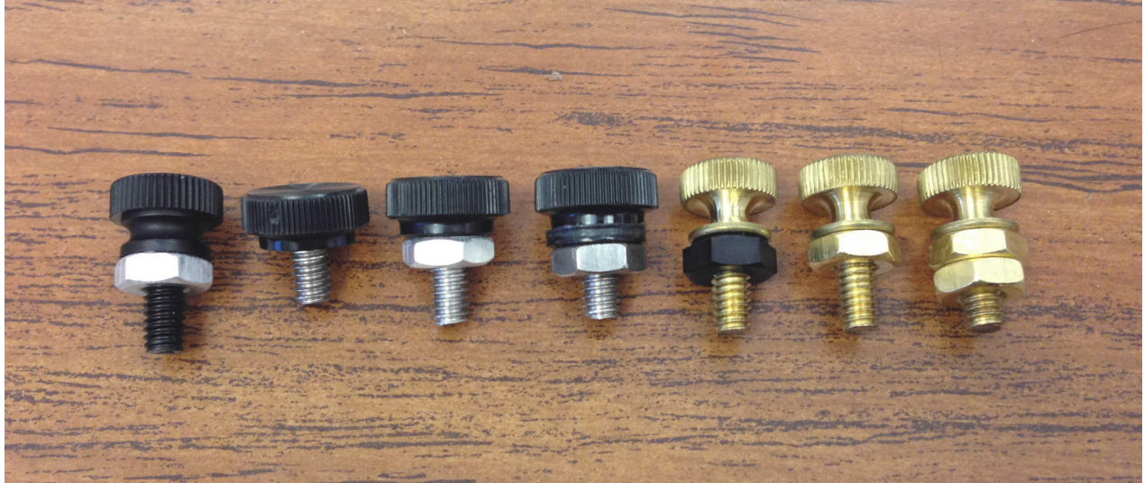
Figure 5. A series of weights you can add to the oscillator, here arranged from lightest (on the left) to heaviest. You should find a pair of each of these in the tray.
